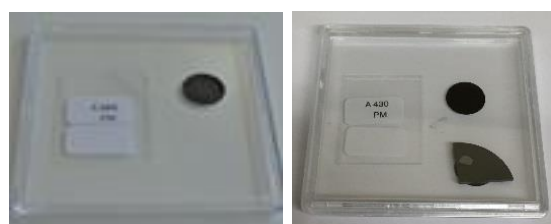
Fig. 2: Sigma-2 adhesive surfaces for light- (glass) and electron microscopy (C-Pad) analysis (left). Sigma-2 adhesive surfaces for light- (glass) and electron microscopy (C-Pad and boron substrate) analysis (right).
