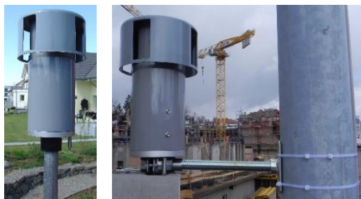
Fig. 1: Sigma-2 passive sampler stuck on a tube (left). Sigma-2 passive sampler fixed with a bracket (right).
